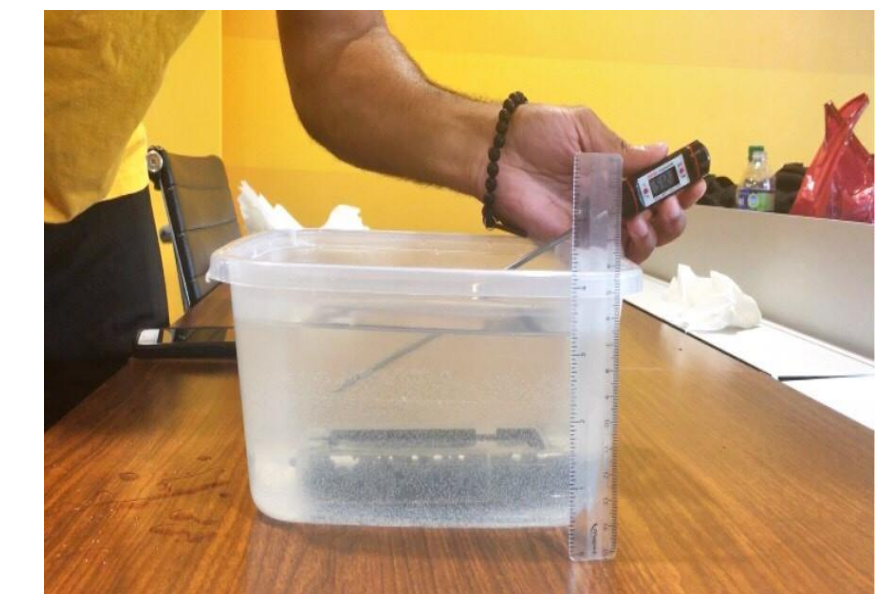
Leak test after drop
