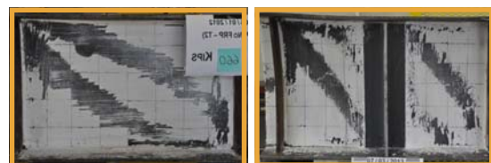
(Left) Bare shear panel, (Right) with SBS
